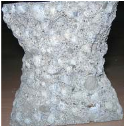
(a) Failure around the aggregate (strength of concrete <30 MPa)
