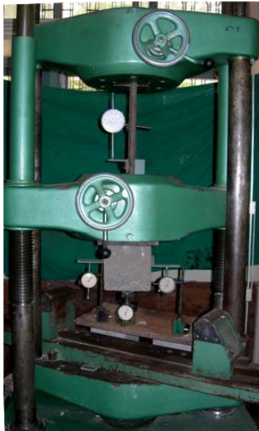
Fig. 4.31 Set up for pull out test
