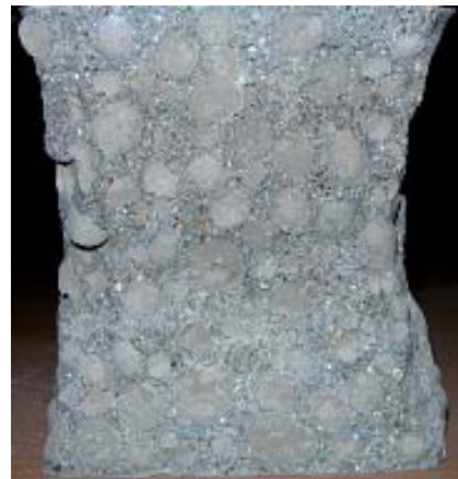
(b) Failure through the aggregate (strength of concrete >35 MPa)
